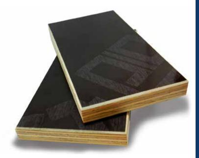
Tulsa Standard Film panels are edge sealed during manufacturing. If you cut boards during the use, it is recommended to re-seal the fresh edges to avoid panel damage caused by capillary penetration of humidity.
